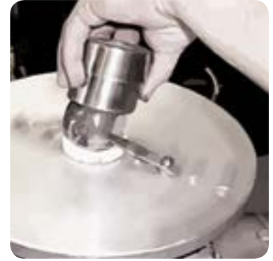
Traditional mate-lapping selectively laps the seat to only one side of the ball, resulting in imperfect spherical geometry and non-uniform coating thickness.
